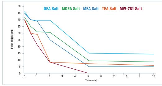
MW-781 is itself inherently low foaming
