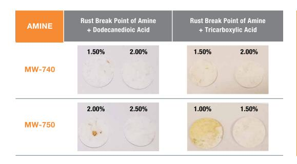
Both MW-740 and MW-750 demonstrate good corrosion inhibition with a tricarboxylic acid and dodecanedioic acid
