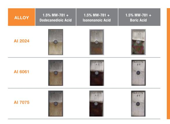
Salts of MW-781 have mild to low staining on aluminum
